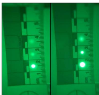
Spots from three different laser beams viewed through the scope of the VRW1B viewer (left), which is optimized for use with sources from 350 - 1300 nm and the VWR2B viewer (right), which is optimized for use with sources from 350 - 1700 nm. Top - 1650 nm at 80 mW, Middle - 1550 nm at 40 mW, Bottom - 1310 nm, 5 mW.
