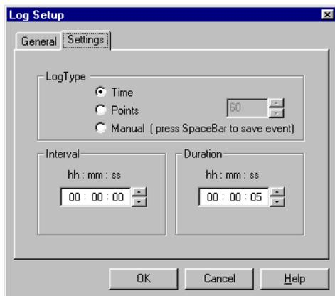
♦ **Interval** Insert the time interval between consecutive measurements. The interval can be set in: hours (h button), minutes (m button), or seconds (s button). After selecting h, m, or s parameters, enter the required value for each parameter using the data entry box.
