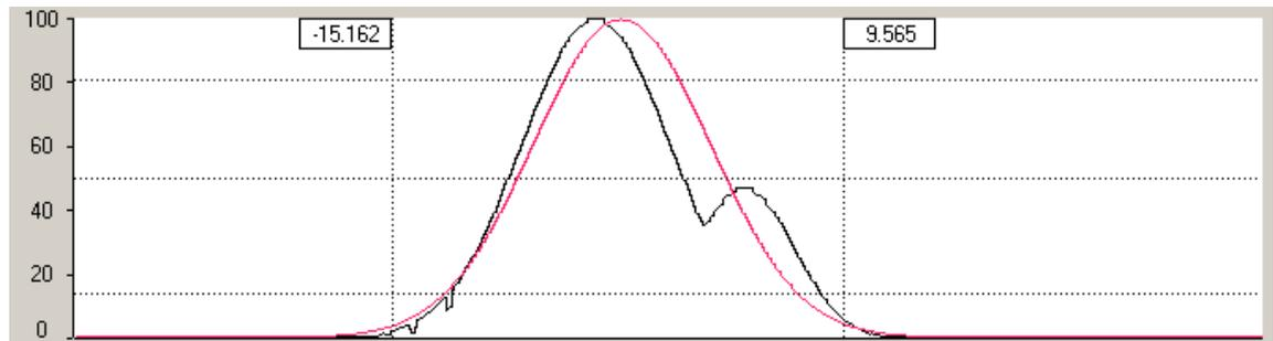
The Gaussian function determines how closely the measured beam profile matches a Gaussian profile. When Gaussian is activated, a Gaussian profile is overlaid on to the actual measured profile in real time. The theoretical Gaussian profile is displayed in red color over the actual measured profile, displayed in white color.
