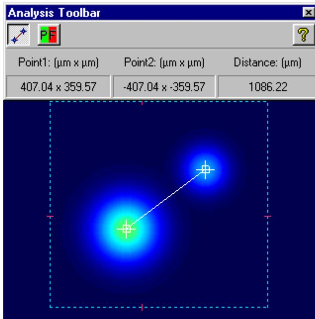
5. Drag the mouse to the second point on the beam image and click the left mouse button. A straight line is drawn between these two points and the line distance calculation is displayed below the Analysis toolbar (see attached figure).
