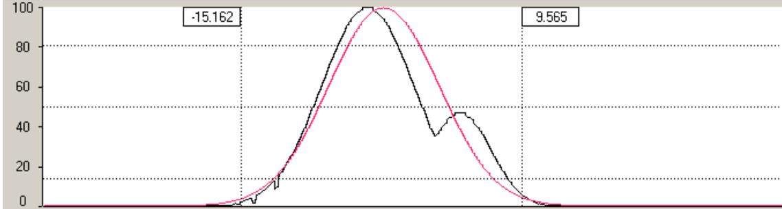
The profiles are calculated and displayed in conjunction with the main ROI, while other two ROI's can be used for presentation of position measurements only! If Gaussian function is On there is a presentation of the Gaussian beam superimposed over the profile in real-time.
