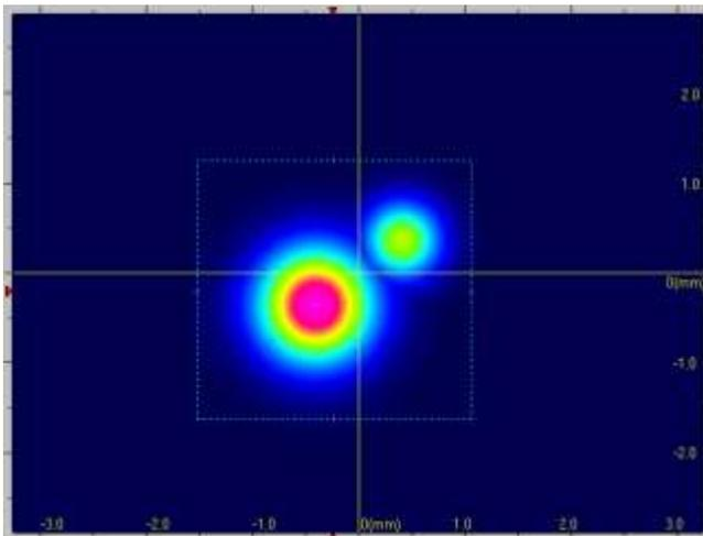
The digitized pixel intensities of the image can be plotted as a 2D contour map in one of two different color scales shown at the color scale bar (color or B/W). When graphics Zoom is enabled scroll bars will appear on the sides of the View Area.
