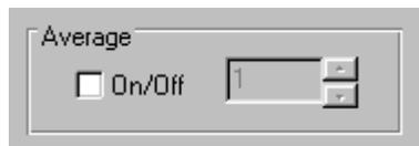
When using a beam with significant amount of jitters, it is sometimes convenient to set Average On.
