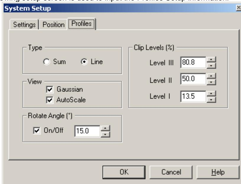
**Type:** Toggle between *Sum Profile* and *Line Profile*. This setting can also be made via the ToolBar. See detailed description in section 8.2.1. Each image is a digital representation of the spatial power distribution across the beam. The numerical value of the profiles width can be viewed in the Profile Measurement Area.
