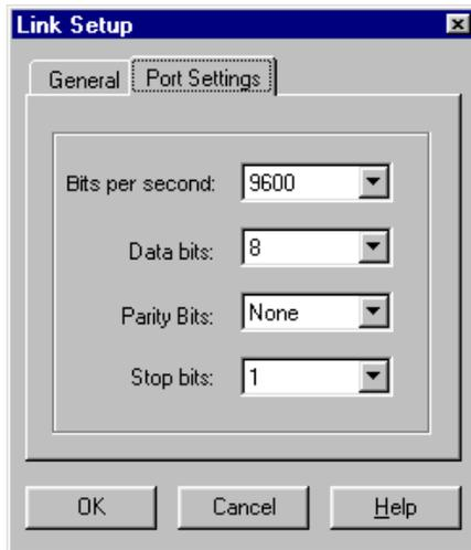
**Port Settings** Tab includes the following four parameters related to the RS232 transmission:
