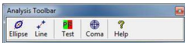
**Ellipse** - Defining a laser beam frequently requires a definition of beam elliptical foot-print and beam orientation with respect to the camera axis. A special function which calculates the best fit ellipsoid to the examined beam is provided by the Ellipse function.
