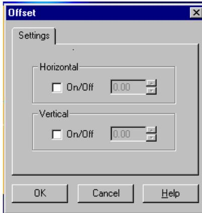
This means that you can have a line profile crossing through a center of gravity or being offset from center of gravity by a certain amount (defined by Offset). The meaning of this feature is that even in an environment where the beam moves the line profile will always stay in the same area with respect to the beam centroid. Set the amount of Horizontal and Vertical offset enabled by 0.1 degrees via this screen.
