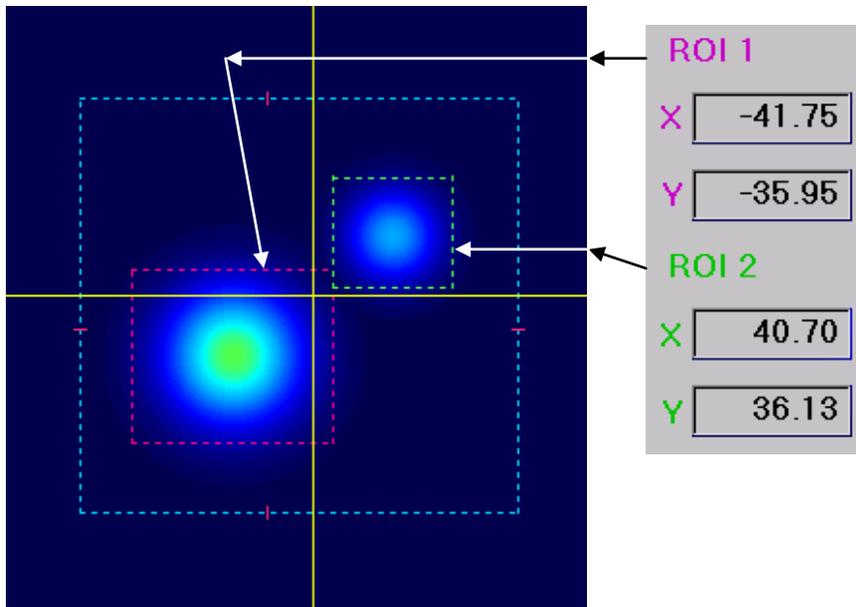
The software calculates the centroid of the beam, which resides inside the ROI area only, disregarding the energy outside of this region. Thus, the result of the beam centroid calculation will be displayed in the appropriate ROI area at the User Area. In case the Radius parameter is set On at the Position Setup – Position tab, then there is an additional calculation and display of the R value, which is the radius of beam centroid with regards to the cross line.
