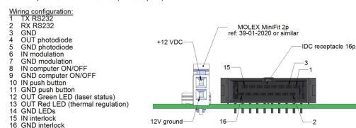
Note: External trigger regime needs a TTL compliant electrical signal on "modulation On/Off" entry from IDC.
