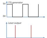
**5 V (or open switch):** the laser is waiting the signal to run
