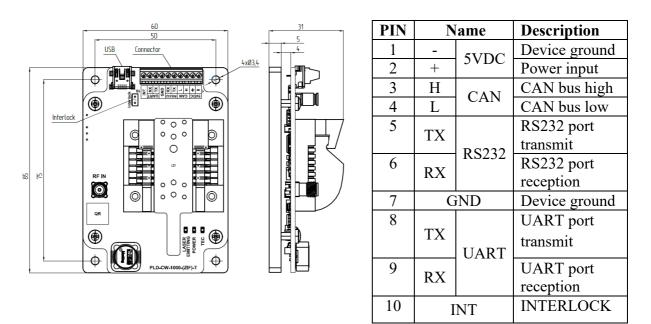
Connect to the external interlock circuit. Open: device is locked, Closed: device is operational. Internally pulled up to 3.3V by 1 k $\Omega$ resistor. Use open collector or dry contact. **Note:** The laser emission can only be started when the interlock circuit is closed
