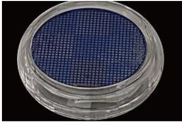
Photograph of imprinted \varnothing 50\text{mm} Indium Phosphide (InP) wafer. All imprinted structures are 20\text{ }\mu\text{m} lines. The protrusion coverage varies from 20% to 60%
