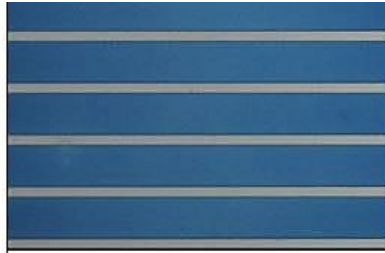
Optical microscope image of 20\text{ }\mu\text{m} lines imprinted on InP. Protrusion coverage is 20%
