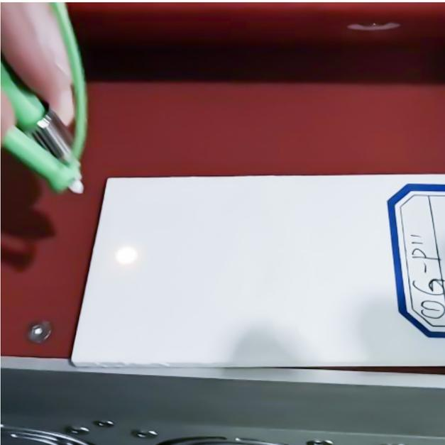
1950nm的激光在1.3W处的测量光斑
